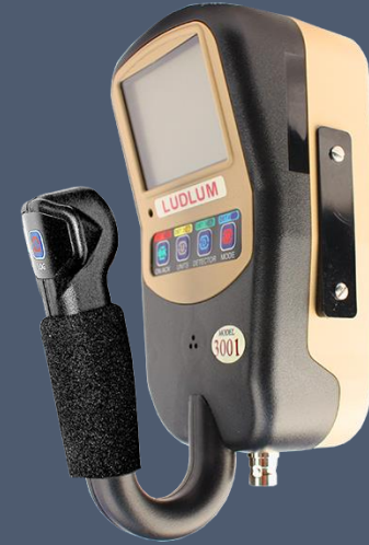
Example of a meter that could be attached to scintillation probe or GM probe
